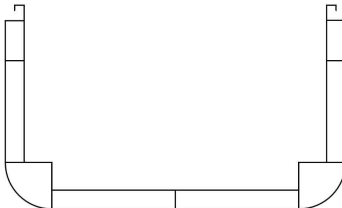
Figure 1 : Container ship of double side skin construction
